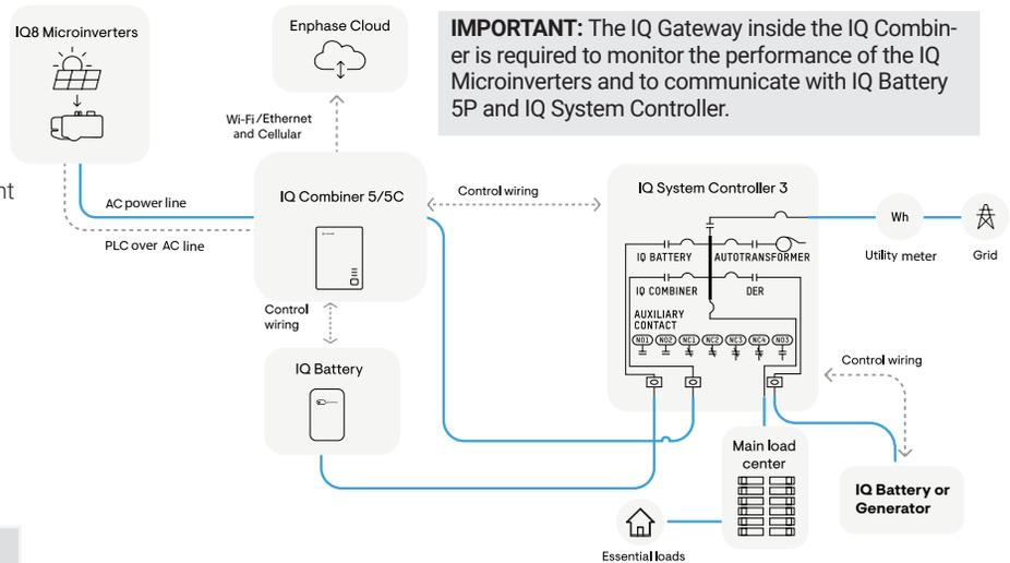
**IMPORTANT:** The IQ Gateway inside the IQ Combiner is required to monitor the performance of the IQ Microinverters and to communicate with IQ Battery 5P and IQ System Controller.
