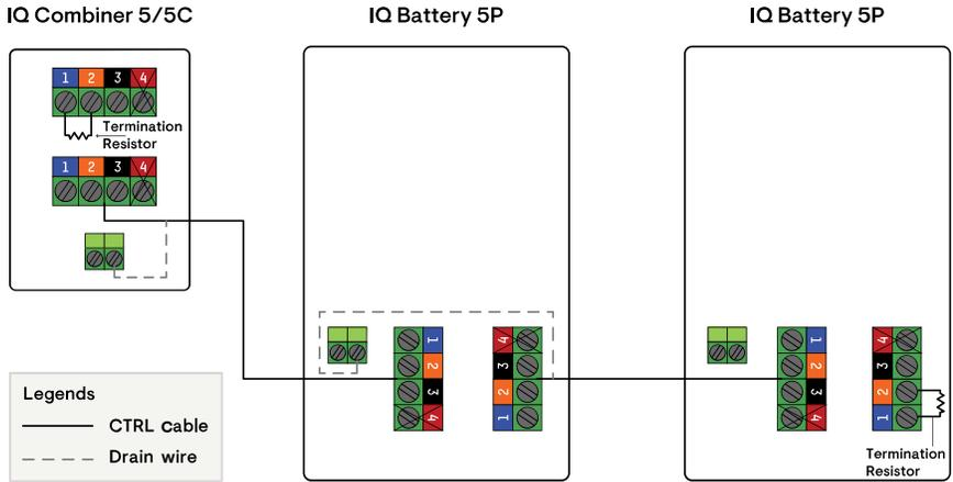
**NOTE:** The total length of CTRL wiring across the system should not exceed 250 feet to ensure the system operates as per specifications.
