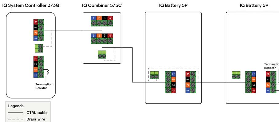
**NOTE:** The total length of CTRL wiring across the system should not exceed 250 feet to ensure the system operates as per specifications.
