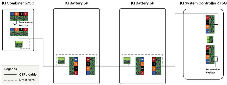
**NOTE:** The total length of CTRL wiring across the system should not exceed 250 feet to ensure the system operates as per specifications.
