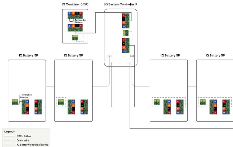
**NOTE:** The total length of CTRL wiring across the system should not exceed 250 feet to ensure the system operates as per specifications.
