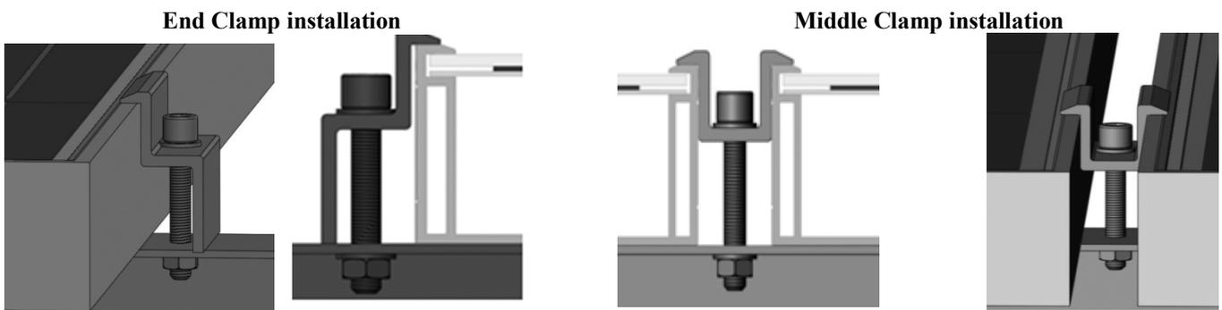
**Figure 2. PV module installed with clamp fitting method**
